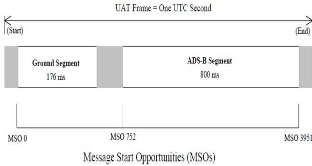
**Figure 11. Ground and ADS-B Segments of UAT Frame**
