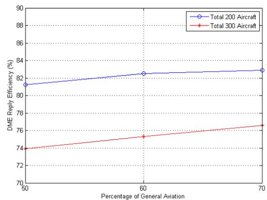
**Figure 13. Expected DME Reply Efficiency wrt. Percentage of GA Users and Total Number of Aircraft within the Service Coverage**
