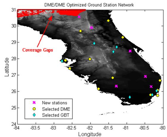
**Figure 8. Optimized DME/DME Ground Station Network**
