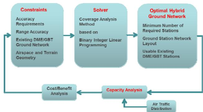
Figure 1. APNT Hybrid Architecture Network Development Process
