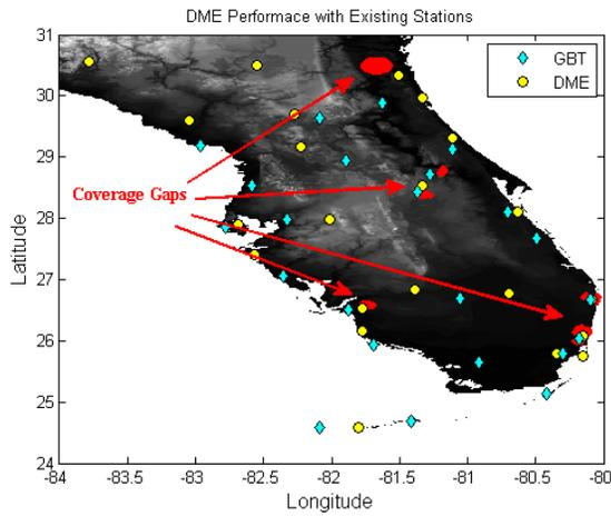
**Figure 5. DME/DME Surveillance Coverage Gaps with All of the Existing DME/GBT Stations**
