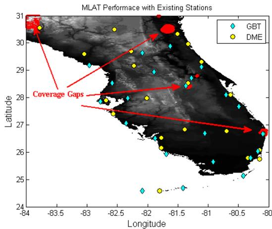
**Figure 6. P-WAM Surveillance Coverage Gaps with All of the Existing DME/GBT Stations**
