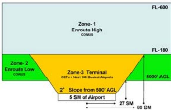
**Figure 3. FAA Airspace Performance Zones (Courtesy of FAA)**
