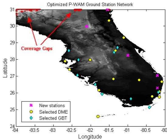
**Figure 9. Optimized P-WAM Ground Station Network**
