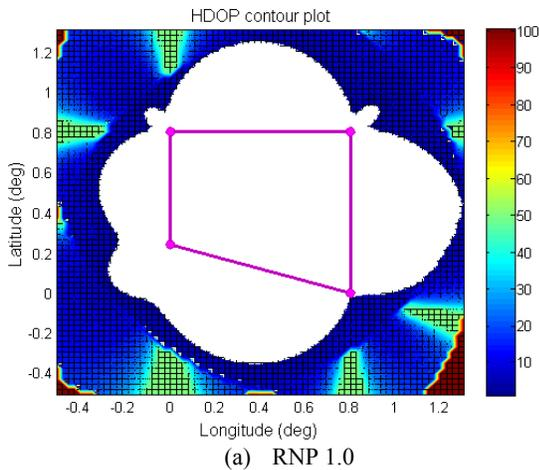
**Figure 2: (a) and (b) Show HDOP Coverage Examples for RNP 1.0. (c) and (d) Show HDOP Coverage Examples for RNP 0.3. Two Station Geometries with  $\sigma_{\text{range}} = 0.085$  nm Are Used.**
