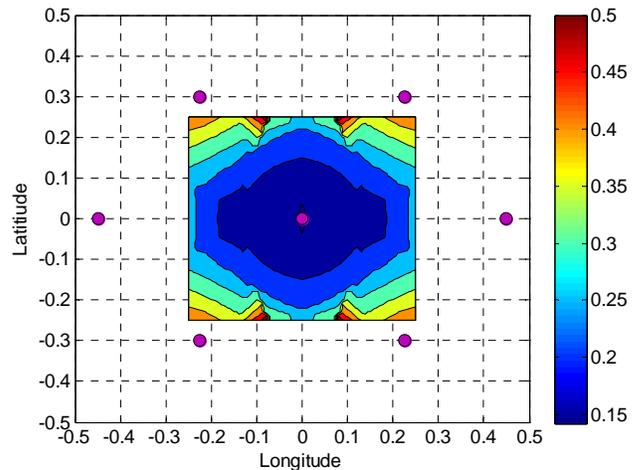
**Figure 13: The Best Resulted Stations (purple circles) of the Iterative Procedure. The 7 Stations Provides the Required HPL Level of 0.6. The Color Map Represents HPL Level. The aircraft is at 500 ft AGL and  $\sigma_{range}$  is 0.085 nm.**
