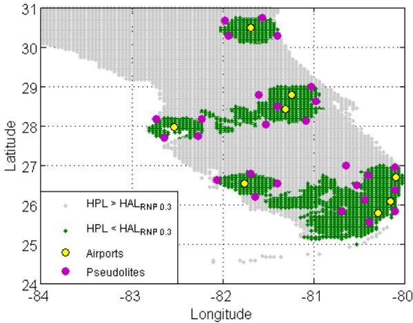
**Figure 17: Station Network with RNP 0.3 Integrity Requirement for the Designated Airports ( $\sigma_{range} = 0.02$  nm)**
