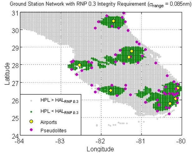
**Figure 15: Station Network with RNP 0.3 Integrity Requirement for the Designated Airports ( $\sigma_{range} = 0.085$  nm)**
