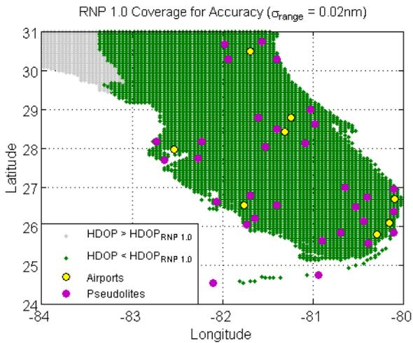
**Figure 20: RNP 1.0 Accuracy Coverage with Updated Station Network ( $\sigma_{range} = 0.02 \text{ nm}$ )**
