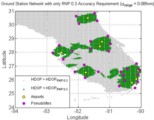
**Figure 14: Station Network with RNP 0.3 Accuracy Requirement for the Designated Airports ( $\sigma_{range} = 0.085$  nm)**
