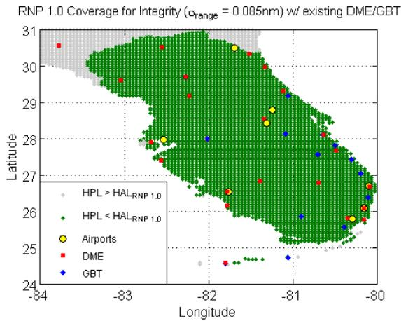
**Figure 5: RNP 1.0 Accuracy and Integrity Coverage in Southern Florida with existing DME/GBT Stations ( $\sigma_{\text{range}} = 0.085 \text{ nm}$ )**
