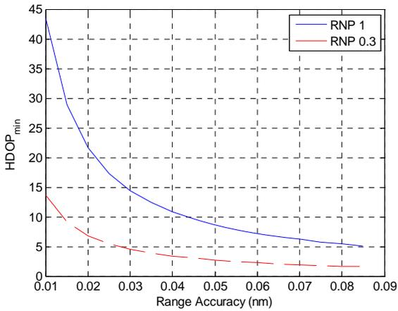
**Figure 1: HDOP<sub>min</sub> vs.  $\sigma_{\text{range}}$  for RNP 1.0 and 0.3**
