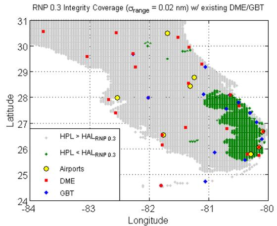
**Figure 7: RNP 0.3 Accuracy and Integrity Coverage in Southern Florida with existing DME/GBT Stations ( $\sigma_{\text{range}} = 0.02 \text{ nm}$ )**
