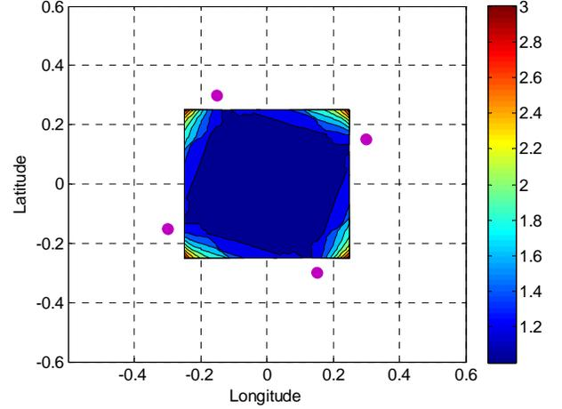
**Figure 9: The Resulted Stations (purple circles) of Initial BILP Formulation. The Color Map Represents HDOP Level. The aircraft is at 500 ft AGL and  $\sigma_{range}$  is 0.085 nm.**
