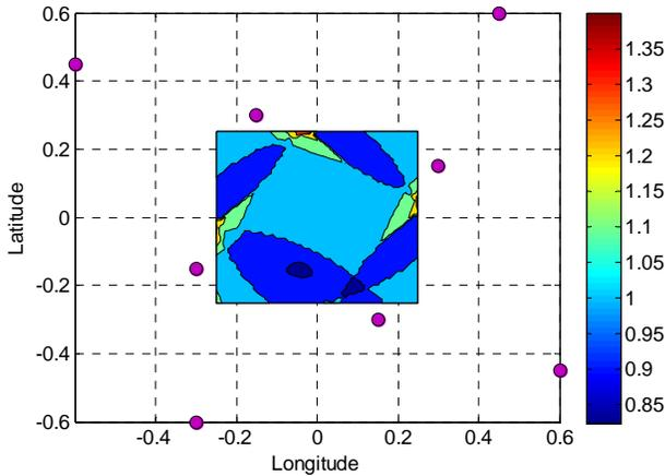
**Figure 10: The Resultant Stations (purple circles) of Updated BILP Formulation. The 8 Stations Provide the Required HDOP Level of 1.67. The Color Map Represents HDOP Level. The aircraft is at 500 ft AGL and  $\sigma_{range}$  is 0.085 nm.**
