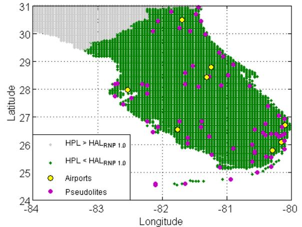
**Figure 19: RNP 1.0 Integrity Coverage with Updated Station Network ( $\sigma_{range} = 0.085$  nm)**
