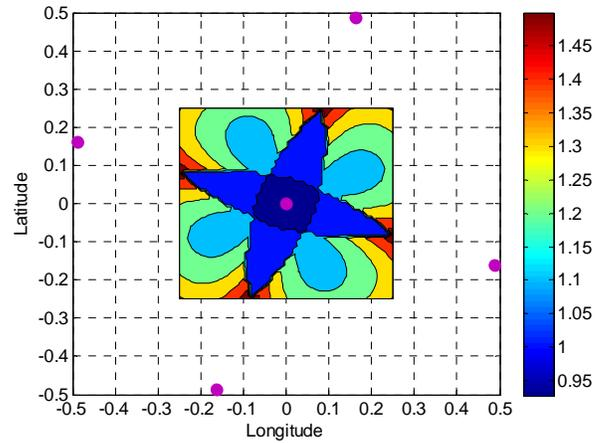
**Figure 12: The Best Resultant Stations (purple circles) of the Iterative Procedure. The 5 Stations Provide the Required HDOP Level of 1.67. The Color Map Represents HDOP Level. The aircraft is at 500 ft AGL and  $\sigma_{range}$  is 0.085 nm.**
