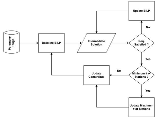
**Figure 11: Flowchart of Iterative BILP Procedure**
