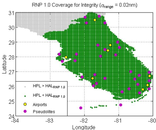
**Figure 21: RNP 1.0 Integrity Coverage with Updated Station Network ( $\sigma_{range} = 0.02 \text{ nm}$ )**
