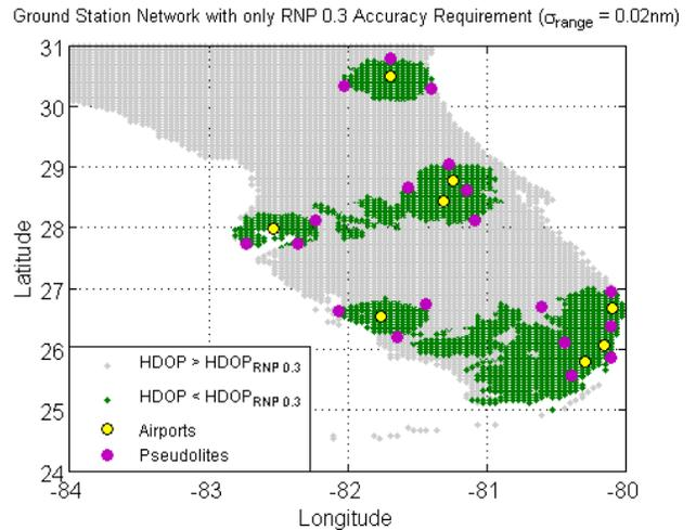
**Figure 16: Station Network with RNP 0.3 Accuracy Requirement for the Designated Airports ( $\sigma_{range} = 0.02$  nm)**
